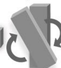
Figure 1 Hold the faces of the gauge block in a cross shape, then firmly slide up and down. Then twist the gauge block back into alignment.
