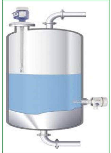
Figure 8. Top and side mounted tuning fork
